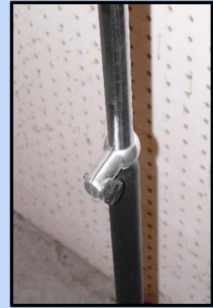
4. Then you decide to add SLIDE STOP . You reset the height and tighten the thumb screw knob to lock the slide tube and PROBLEM SOLVED!
